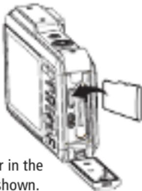
Insert the card with the marked corner in the direction shown.
